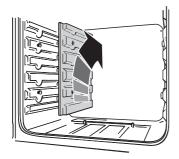
Once the linings are removed, the oven enamel interior can be cleaned.
